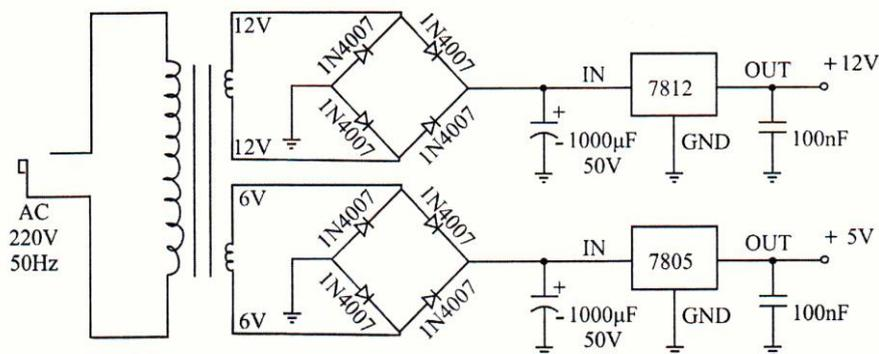
Fig.5 Regulated power supply circuit
