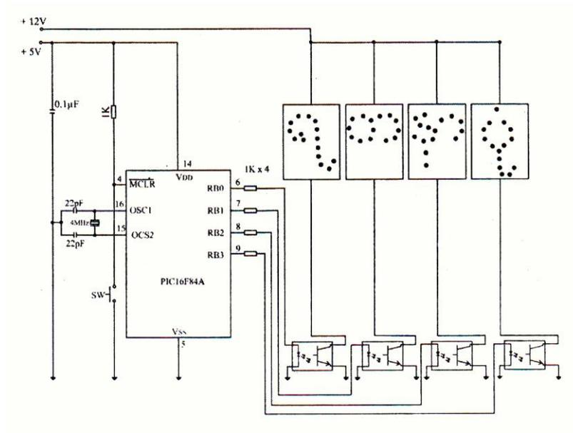
Fig.6 Circuit diagram of “A Microcontroller Based LED Display Board”
